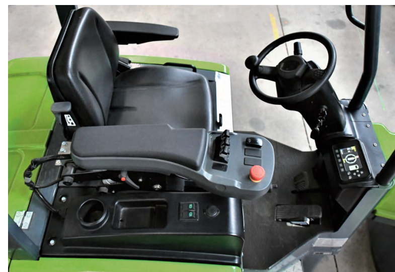
Options: Electric proportion integrated handle, easier operation and more accurate
