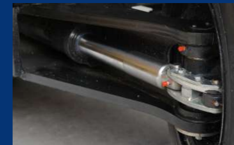
02 Heavy duty steering axle with tapered bearings.
