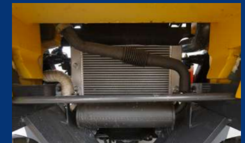
03 The combined radiator with serpentine wave and optimized heat dissipation channel enhance the heat dissipation capability to keep engine reliability even in heavy-duty applications.
