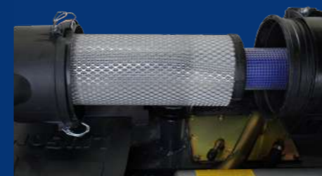
04 Dual air filter to adapt to dust conditions, prolong the service life of the engine.
